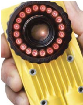
LED array provides economical bright light for many applications.
